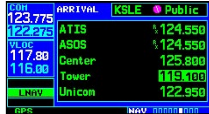
Selecting a frequency on the NAVCOM page.
