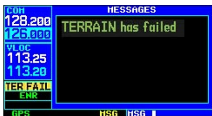
“TERRAIN has failed” message
