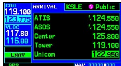
Swap the standby COM frequency into the active Com frequency location.
